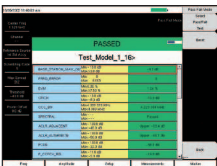
The UMTS Master offers a clear Pass/Fail display for quick evaluation of a Node B base station.
